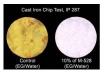
M-528 provides corrosion protection for hydraulic fluids in harsh subsea environments. The image shows M-528 evaluation in an Ethylene-glycol water solution, IP-287.
